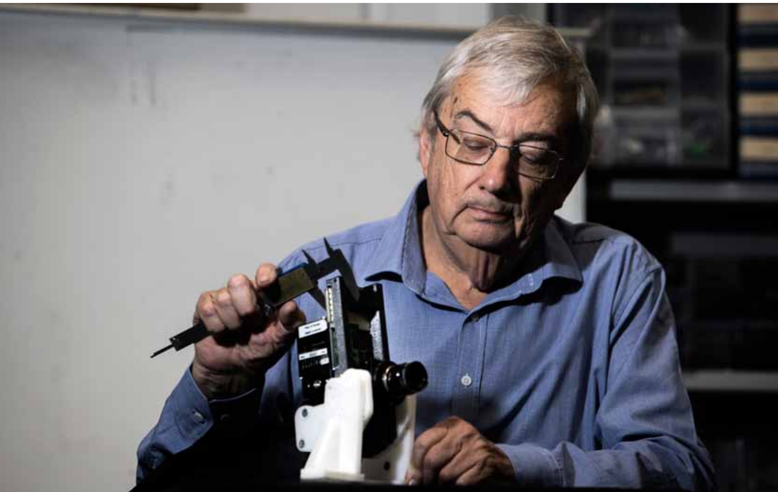
Dr Terry Cocks of HyVista Corporation with the C-SASS sensor. C-SASS can change its look angle, it has a very low signal to noise level and can be mounted on a wide range of aircraft including drones. The C-SASS sensor is part of DMTC's collaboration with HyVista Corporation, UTS and DSTG. More information on the C-SASS project can be found above.
