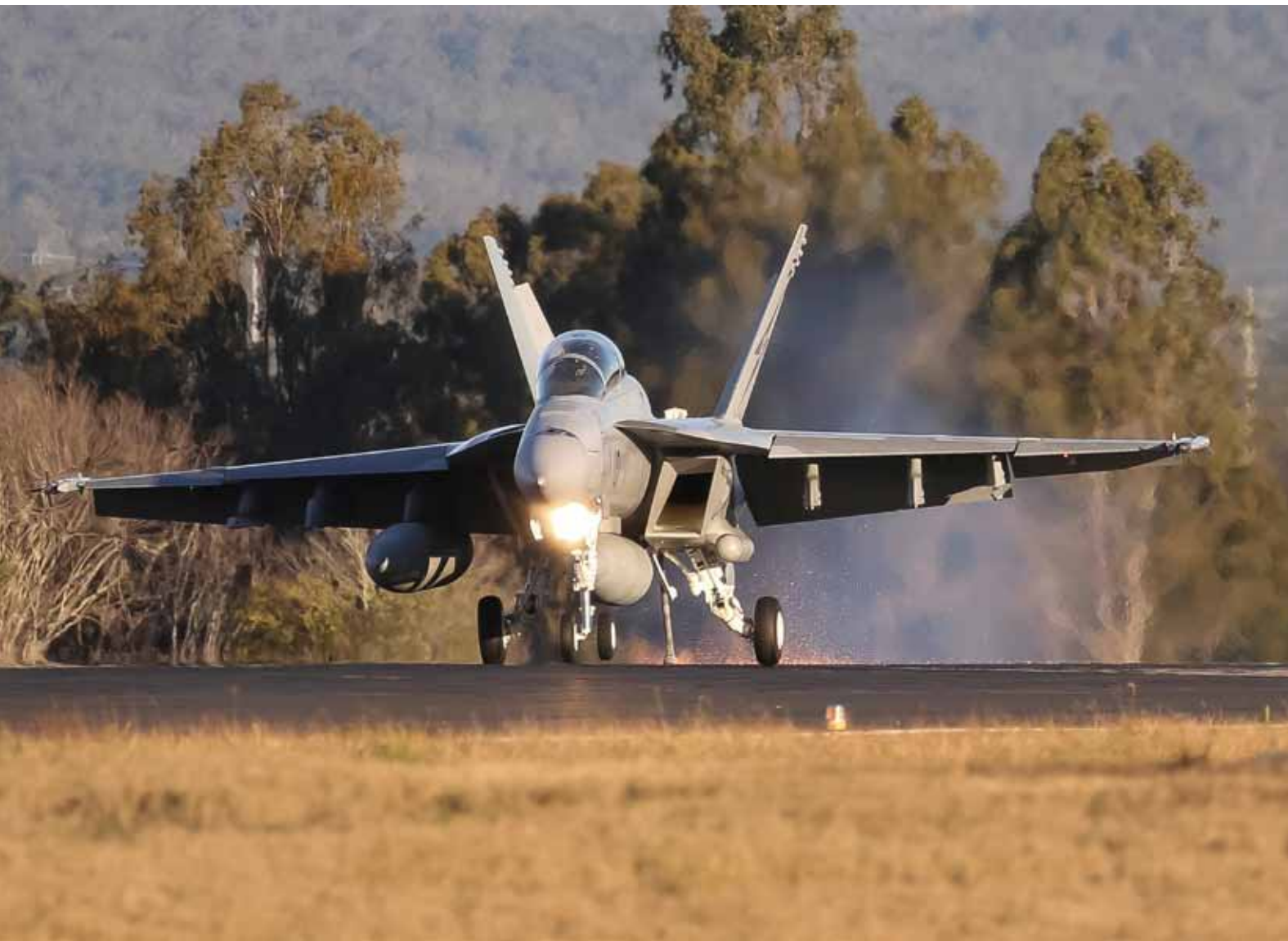
A Royal Australian Air Force F/A-18F Super Hornet aircraft lands while engaging the aircraft arrestor cable at RAAF Base Amberley, Queensland. The RAAF's aircraft arrestor systems are lifesaving devices utilised in fast jets in the event of an emergency. Arrestor hooks are an example of the non-structural aircraft components that can be repaired, rather than replaced, using laser additive deposition (LAD) techniques.
